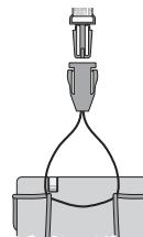
Pull the loop of the band over the clip, slide the pushbutton to the desired length of the band and put the band around your neck. By unlocking the snap connection (
